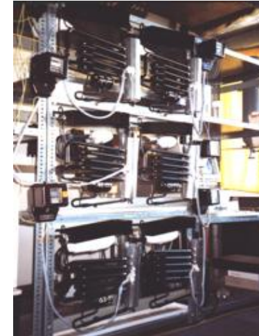
Absorption-refrigeration aggregates (Dometic, Tadiran, Sibir, Sanyo) in a lab of the IFT, University of Siegen icy bulbs around evaporators clearly can be recognized.
