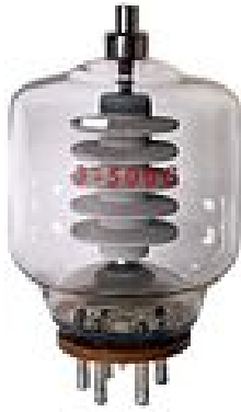
Radio valve, 500 W graphite anode
