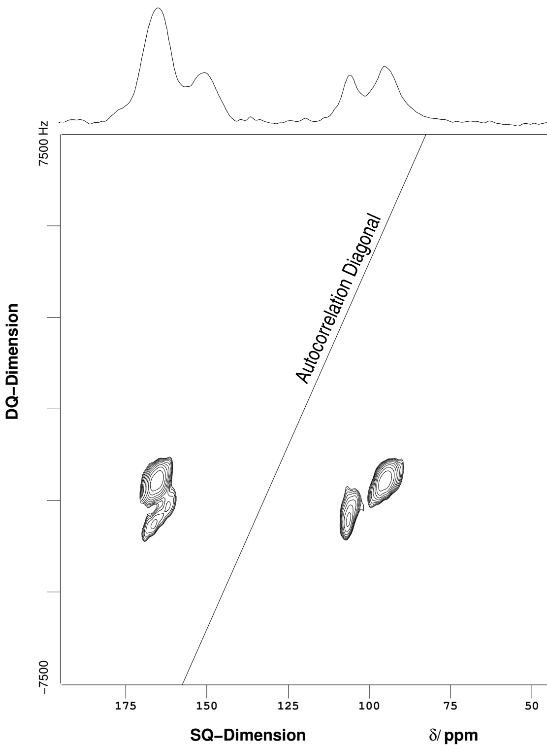
Figure 6: 2D double-quantum filtered correlation spectrum of poly(carbonsuboxide) ( sample II ) using the through-bond dipolar coupling for double-quantum coherence excitation (pulse-sequence A, figure 2).
