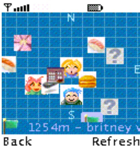
Figure 1: The radar interface that represents the local map of the game around the player (whose icon always appears in the centre of the screen) in an area of four square kilometers. The other players and geo-localized virtual objects appear on the map. The 'closest Mogi-friend' is indicated at the bottom of the screen, with the distance even if it is more than 2 kilometers. This functionality was added by the designers to facilitate the 'onscreen encounters' discussed below.
