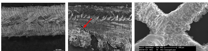
Fig. 3. Grinded cross sections of (left) a vertical strut and (centre) a diagonal, 45°-strut with melting deposit and cracks at the lower strut side. (Right) BCC-node from top.
