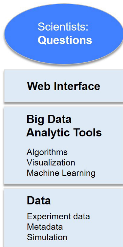
Figure 3: Web working environment with tentative labeling Scioogle enabling scientists to answer their scientific questions by accessing research data, developing and applying Big Data Analytic Tools, having the computing power available for data processing, and visualizing the results.
