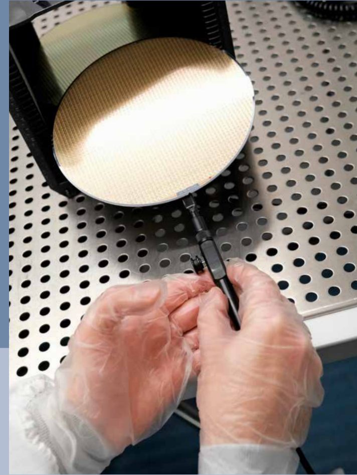
Dr. Christian Karcher charakterisiert am Labormessplatz pmd-Sensoren. Dr. Christian Karcher characterizes pmd sensors at a laboratory measuring station.
