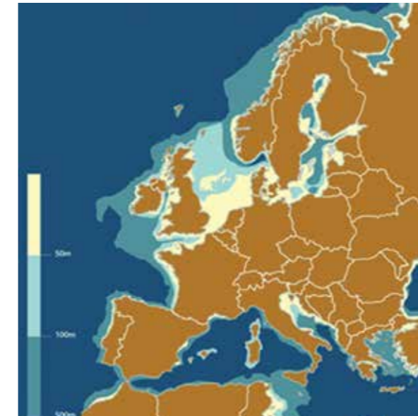
Simplified pan-European bathymetry and wind speed maps, highlighting the limit area available for wind energy development in shallow water vs. areas for which deepwater solutions are required. (Source: Acciona, 1 Tech)
