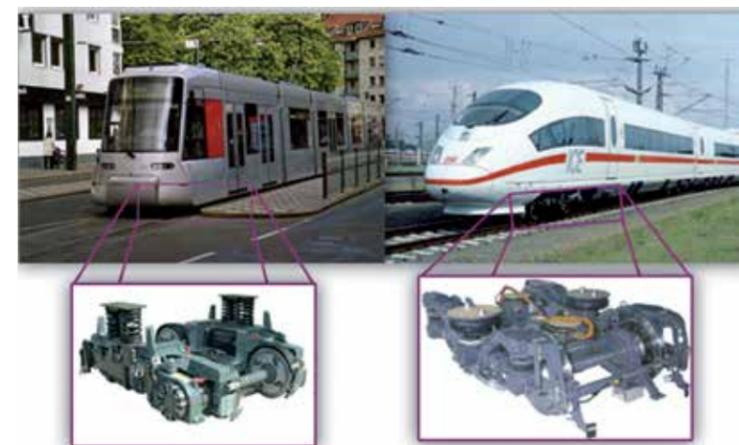
Figure 1: The Bogie as a link between superstructure of the train and the rail
