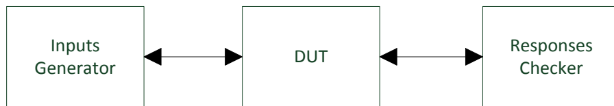
Figure 50: Overview of the basic Verification Concept
