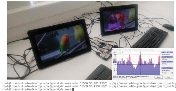
Figure 12: Regulating video streaming quality using NetGuardXt.
