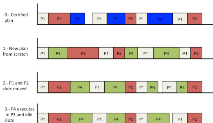
Figure 4-9 Comparison of alternative scheduling plans once P3 is removed from the certified scheduling plan
