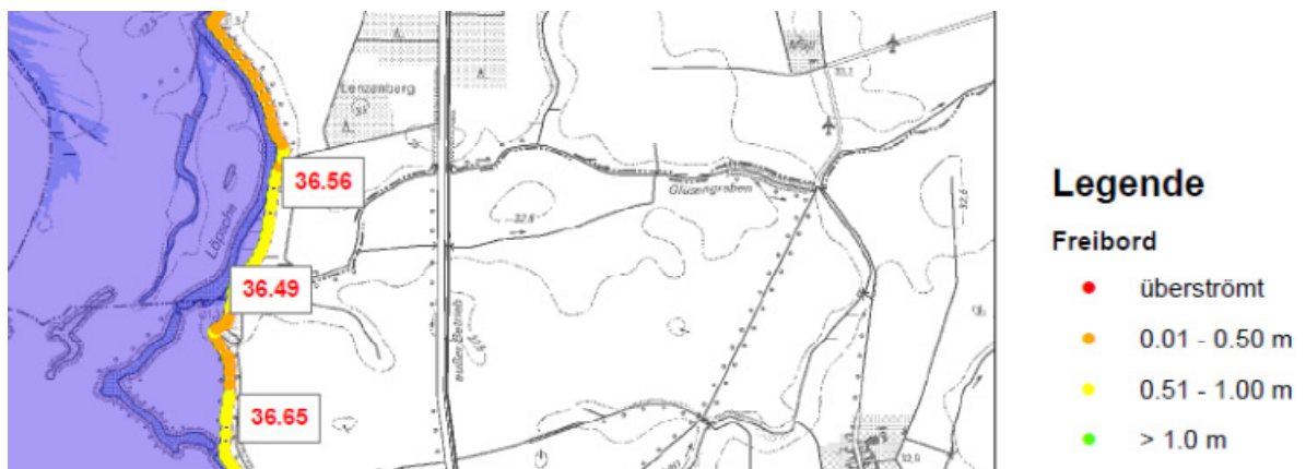
Figure 5: Map with classification of freeboard along Elbe dike by scenario with a return period of 200 years (LHW)
