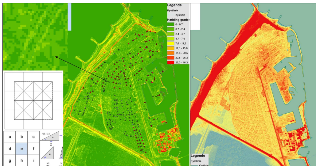
Figure 9: General elevation pattern (right) and surface slope map. Manhole covers are either in areas with slope gradients <0.7^\circ (green dots), typically in the middle of roads, or >0.7^\circ (red)
