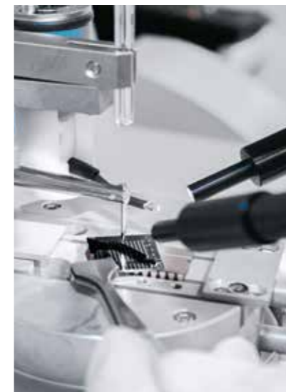
Graphen-Sensor im Bonding Tool Graphene sensor in the bonding tool
