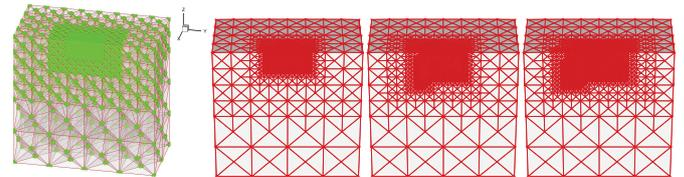
**Fig. 3.** Initial mesh with sampling clusters around mesh nodes (left). Adaptive mesh refinement, which is directed by the 2nd invariant of the Green strain tensor, enables an unbiased dislocation evolution by fully atomistic resolution in regions involved.
