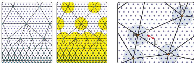
**Fig. 1.** Crystal subject to FE-discretization (left) and with cluster-atoms for energy sampling (centre). The method is fully nonlocal including interactions across clusters (right).
