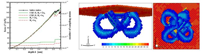
**Fig. 2.** Force-displacement curves show quantitative agreement of CQC-E with MS in both the elastic branch and the force-drop indicating dislocation nucleation (left). Dislocation microstructure (centre and right) below the indenter in agreement with MS.
