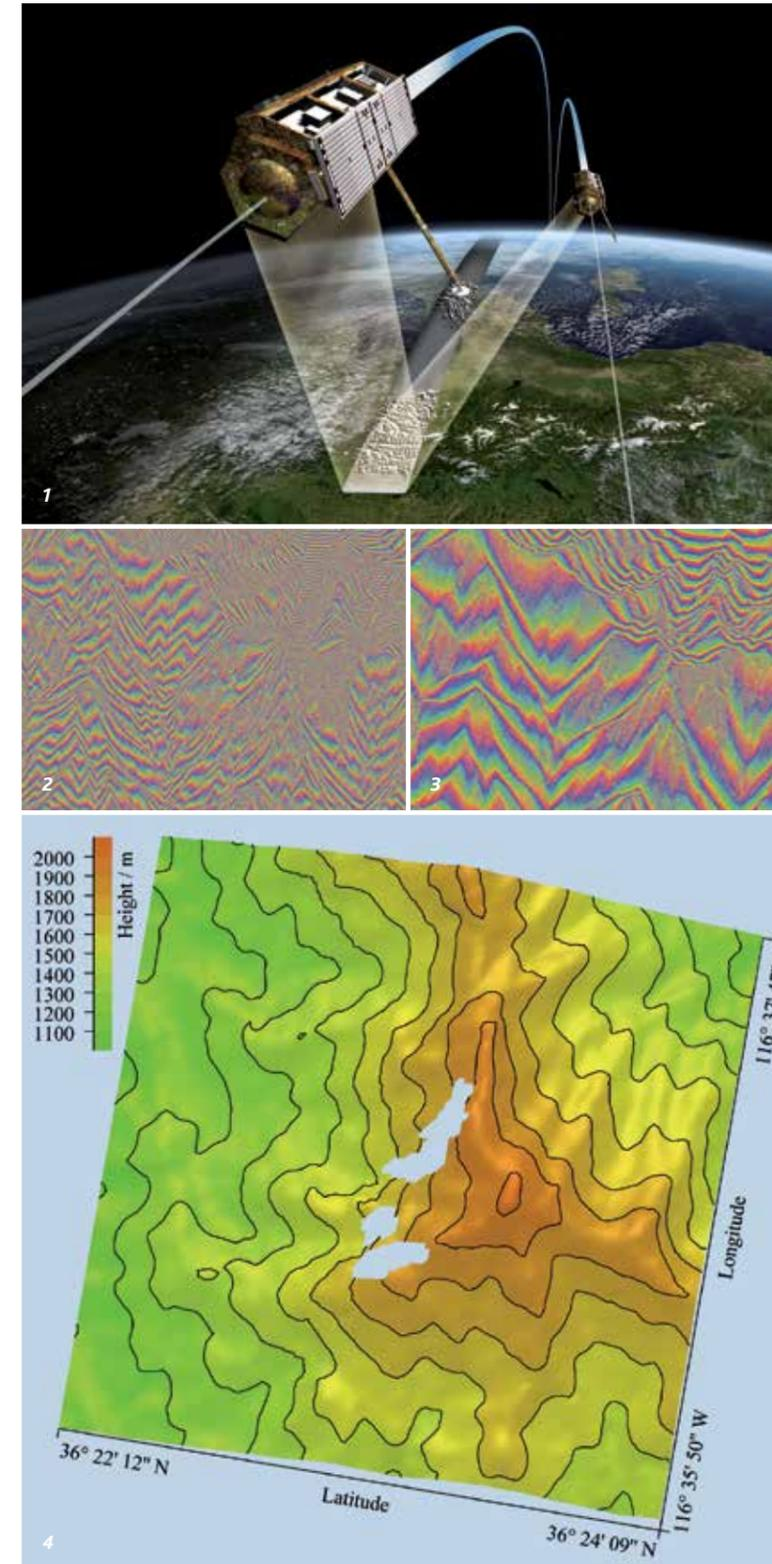
Fig. 1. TanDEM-X configuration. The radar satellites TerraSAR-X and TanDEM-X are flying in a close formation. In the standard bistatic mode, one satellite illuminates the scene while both satellites receive the radar echoes. Image: DLR, CC-BY 3.0
