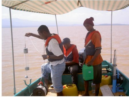
Figure 4.5: Water sampling from fixed monitoring station.
