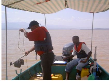
Figure 4.3: Grab sampling of lake bed sediment from predefined sampling site.
