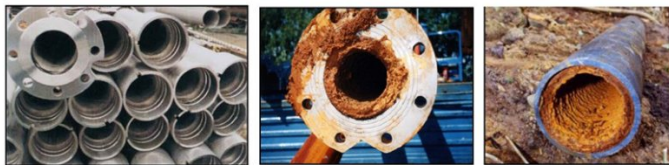
Figure 6.14: a) New rising mains; b) Rising main with ochre deposits; c) Old ground pipe laying
