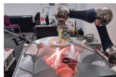
Figure 5: Current STIFF-FLOP manipulator operating inside a 2:2 scale phantom environment of the abdominal area.
